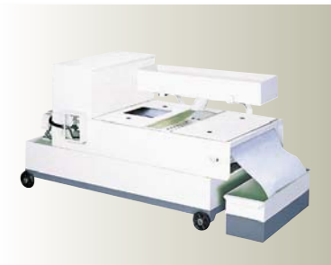
COOLANT SYSTEM WITH AUTO PAPER FEEDING DEVICE (With 1 Roll of Paper) B17-0301 Volume: 120L Paper feeding motor: 25W Pump: 1/8HP Coolant Capacity: 20L/min Space: 57"x24 3/8" (1450x620mm) Height: 30"(760mm)
