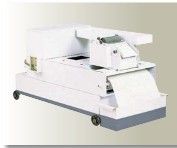
COOLANT SYSTEM WITH AUTO PAPER FEEDING DEVICE & MAGNETIC SEPARATOR (With 1 Roll of Paper) B17-0302 Volume: 120L Paper feeding motor: 25W Pump: 1/8HP Coolant Capacity: 20L/min Space: 57" x24 3/8" (1450x620mm) Height: 30" (760mm)
